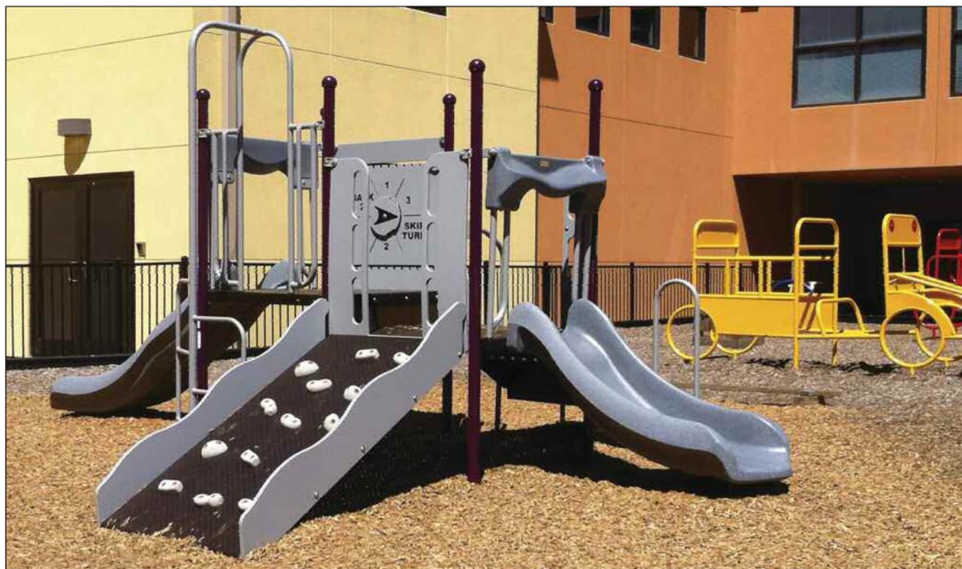
Engineered wood fiber provides excellent fall protection but requires more frequent maintenance.
