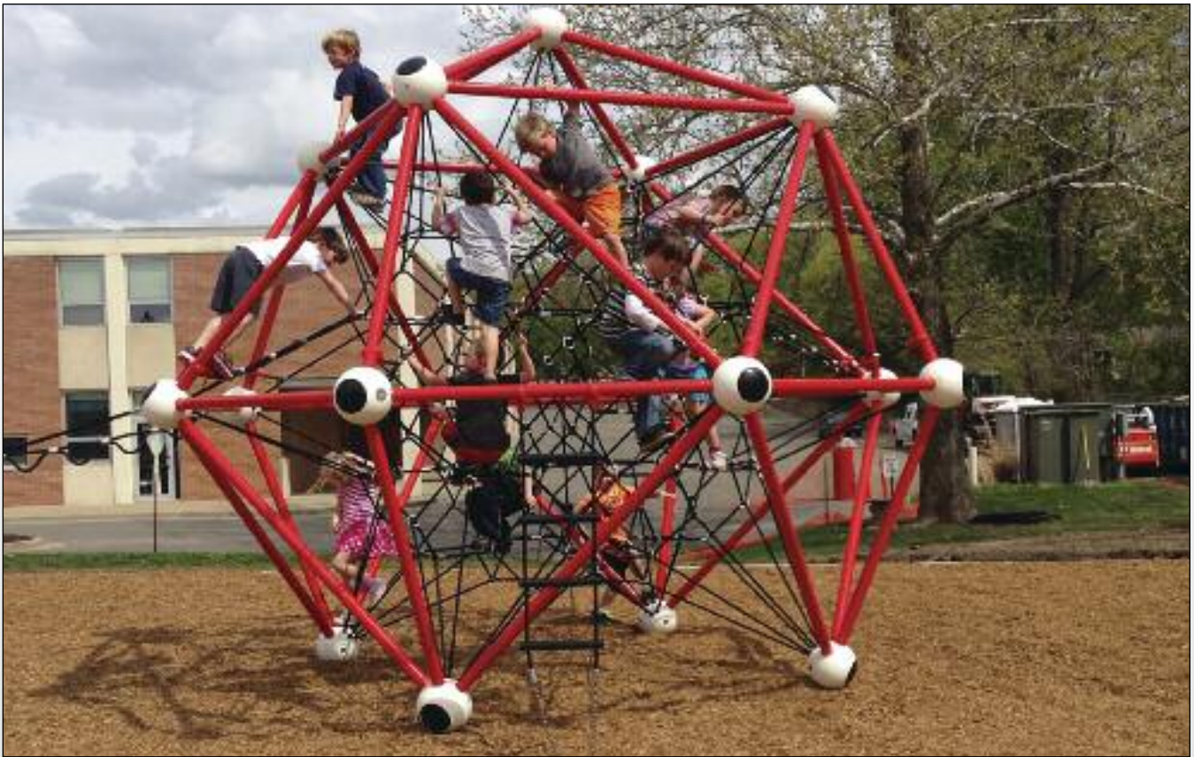
At Cure of Ars Catholic School in Kansas, engineered wood fiber provides excellent fall protection and a natural look.
